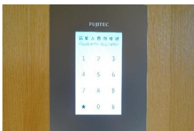
Users can register floors in the elevator hall when going to other than those previously registered
