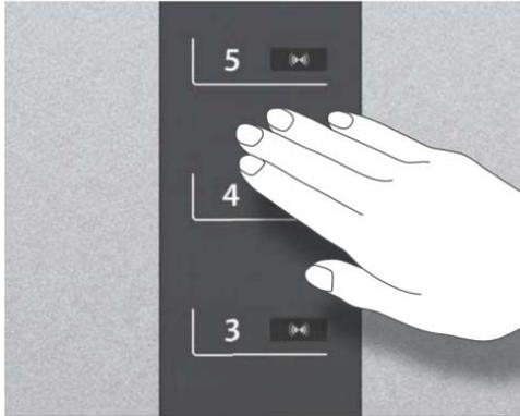
Riders sweep hand over an infrared sensor to call an elevator car and indicate destination without touching any buttons
