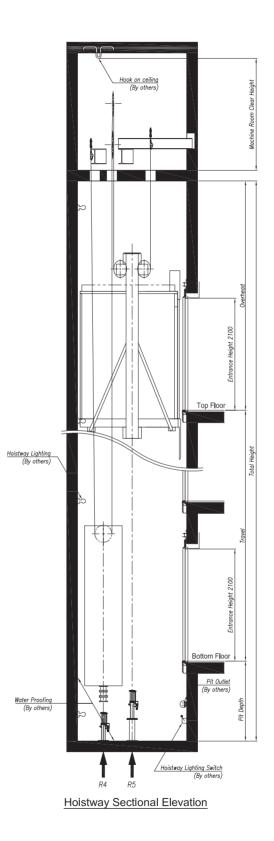
Note: 1. The above dimensions may be affected by the selections of elevator specification and the given hoistway size. 2. The above overhead is based on the Travel of 40 m or less. 3. The above overhead is based on the ceiling design of CT-GS01. The isoamerican of the actual boistway with the above required hoistway size affect the overhead.
