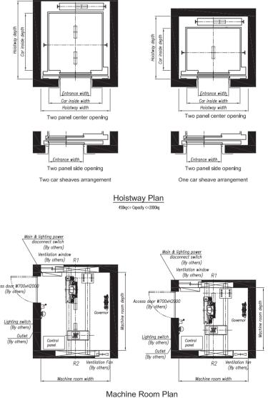
Note: When the elevator speed is 3.0 m/s and the machine room width is the same as the hoistway width, it is required to cut out the machine room wall to prevent interference with governor machine.
