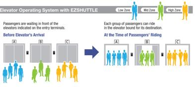
In an elevator operating system with EZSHUTTLE, passengers are required to register their destinations at the elevator floors rather than conventionally registering them inside the elevator. The EZSHUTTLE system then guides passengers to their assigned elevators, which will have been selected to minimize the number of destination stops
