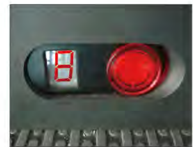
Fault Display for S and F Type
